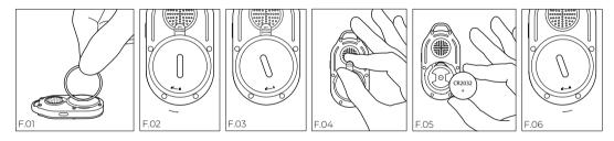
This product includes two replaceable CR2032 batteries with a lifespan of 20 months. The batteries are pre-installed inside the product and protected by a paper sheet. To install them:
